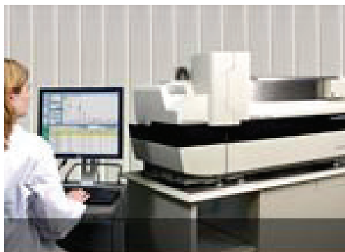
Figure 4 The Life Technologies FlashQuant™ system couples a MALDI ion source with a triple quadrupole mass spectrometer
