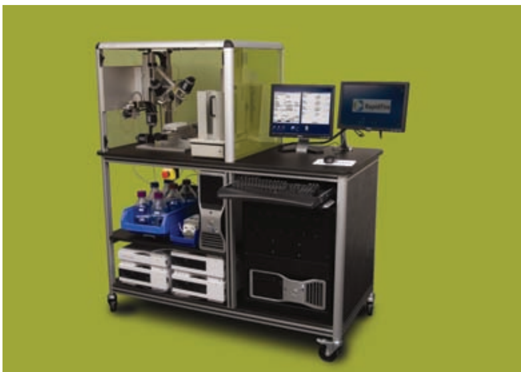
Figure 5 BioTrove's RapidFire System directly couples SPE purification to a mass spectrometer for high throughput analysis
