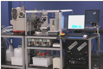
Figure 1. Biotrove screening technology platform consisting of Biotrove system interfaced to Applied Biosystems API4000 triple quadrupole mass spectrometer
